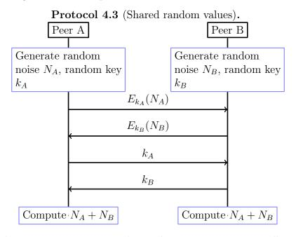
To generalise this to n peers, we ensure that each peer waits to receive all encrypted noises before transmitting their decryption key.
