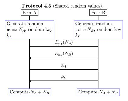
To generalise this to n peers, we ensure that each peer waits to receive all encrypted noises before transmitting their decryption key.
